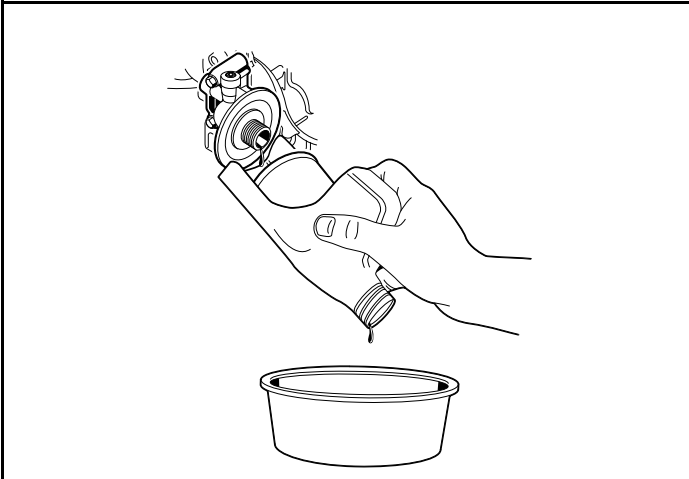
Figure 10-6 Remove Engine Oil Filter
